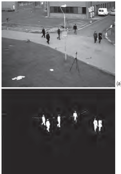
Figure 2. Background subtraction: (a) Input image, frame 332 of PETS 2009. (b) Target detection results, six blobs formed from the pedestrians on the scene. Also, some clutter is detected.
