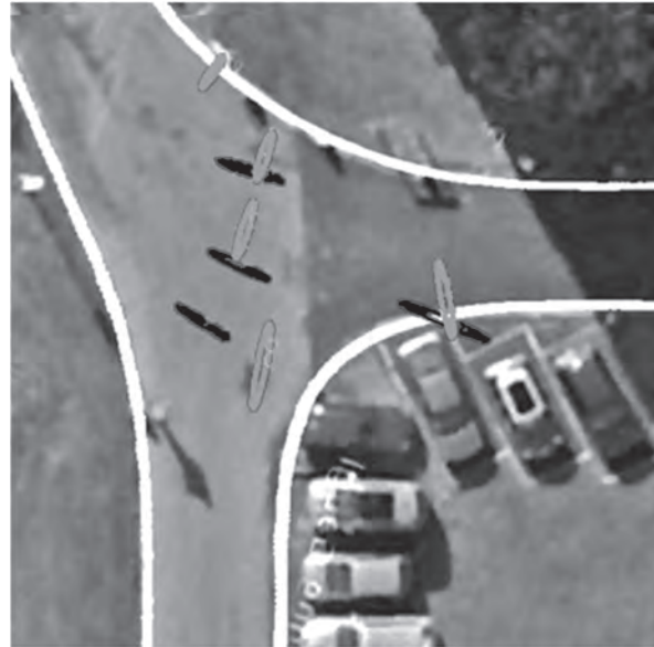
Figure 3. Data association: Projected estimates. The ellipses depict the variance of the projected single-target estimators onto the ground plane. Colors correspond to the cameras IDs (black for view 1 and gray for view 2). For each view we want to associate at most one of these "observations" to particles on the ground.
